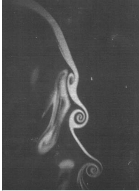
FIGURE 11. LIF longitudinal visualization of the jet flow at R \approx 2 .
