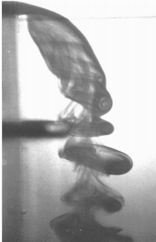
FIGURE 12. Longitudinal view of the jet flow mixed with blue dye at R \approx 2 .
